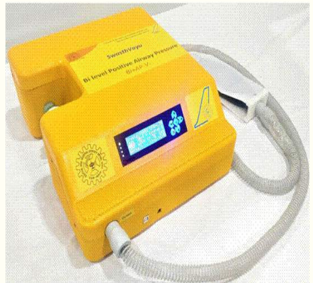
Swasth Vayu BiPAP Machine in Auto Test mode with Test Lung
