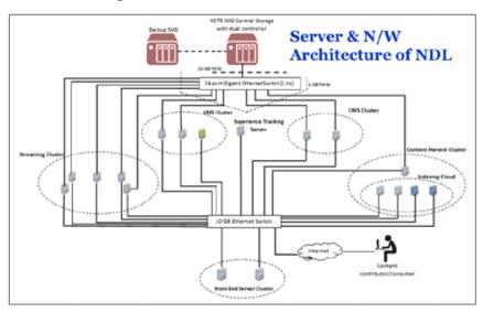
Figure 6: Server and Network Architecture of NDL
